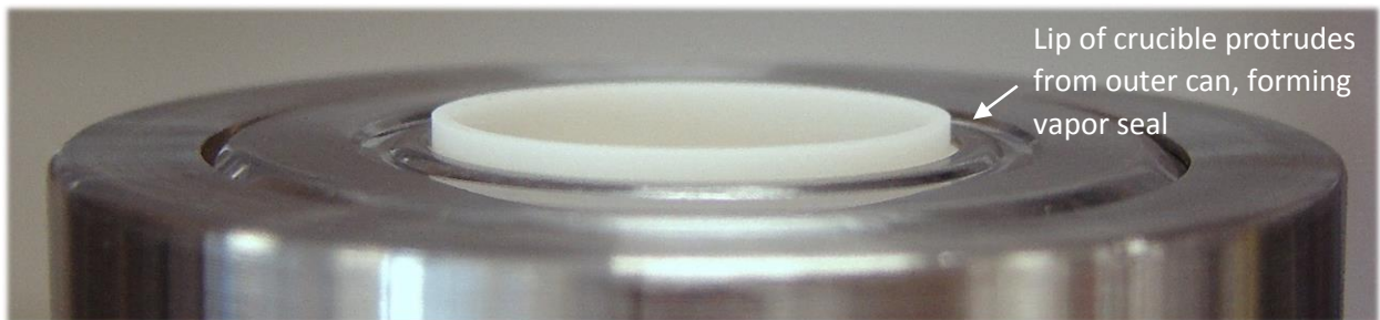
Figure 6: For lipped crucibles, ensure that the lip protrudes from the vapor shield outside the furnace, indicating the crucible is centered and the vapor seal has been properly formed.
