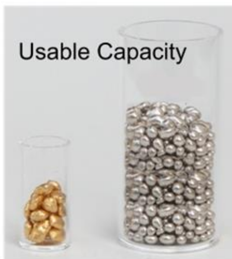
Figure 8: Recommended crucible fill level for non-subliming materials is \frac{3}{4} full.
